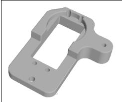
3D print one gripper servo mount per drawing Relic.11M
