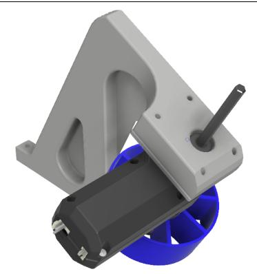
Attach the motor mount to the stand using 1.25" 6-32 bolts.
