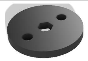
Using ABS, 3D print four wheel washer adapters per the drawing - Intake.3.M.
