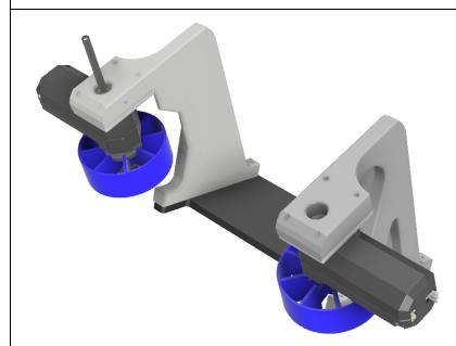
Using 6-32 bolts, attach the mounts to the baseplate of glyph collector.
