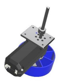
Slide the axle into the axle slot on the motor.
