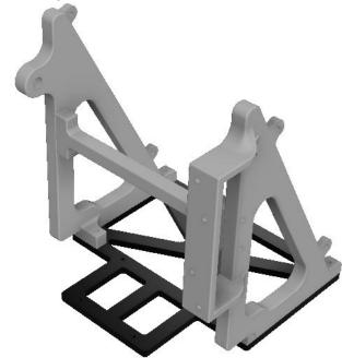
Attach long I-beam support between right and left support.
