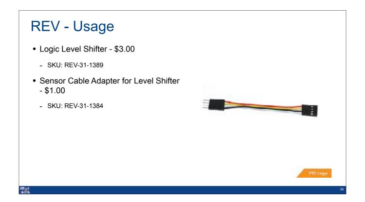
Because the level shifter has a different pin-in on one side than standard modern robotics sensors, REV sells this city little adapter that changes the pins to match that of the level shifter. The other option of course is to just pull one end of the sensor cable apart and rebuild the connector with the pins in the right order. \*Next\*
