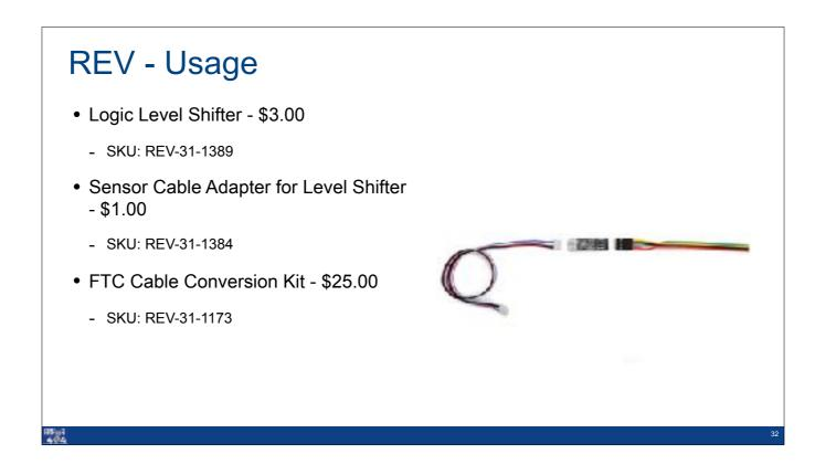
REV also sells a cable conversion kit. The kit comes with 3 Level Shifters, 3 REV Sensor Cables, 1 Adapter Cable for the Level Shifter, 4 motor adapters (converts the Anderson Two Pole cable to the REV Motor Type Cable — lets you use your Pitsco and andymark motors with the REV Hub).
