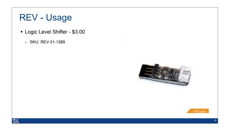
So Here's the Level Shifter. It is required to change the voltage between the REV Hub and third-party sensors. This is because, as I stated earlier, the REV Hub and REV Sensors use 3.3 volts and most other sensors use 5 volts or there about.
