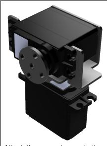
Attach the second servo to the servo mounting bracket.
