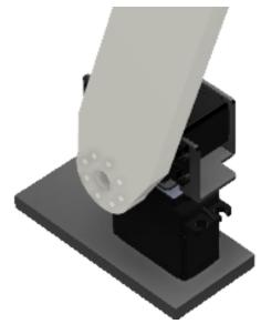
Attach the sword to a servo horn and then attach to the servo per drawing Sword.1.E
