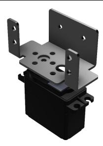
Attach the servo mounting bracket to the servo horn as shown and then attach to the servo.
